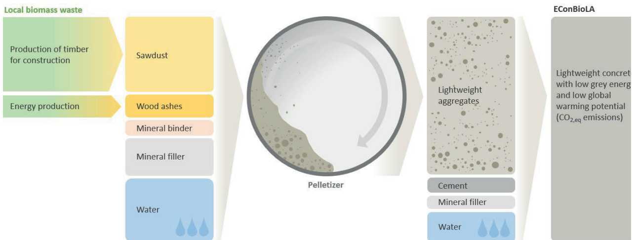
Figure 2. Fabrication process of lightweight aggregates and lightweight concrete
